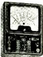
MODEL 103 (1000 ohms per volt meter)
