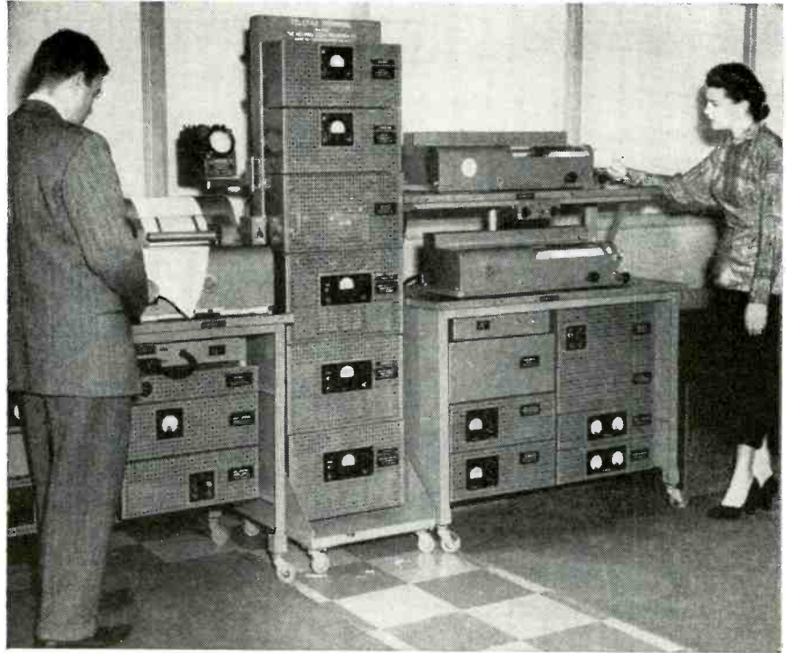
New high-speed facsimile equipment. The transmitter is at right, receiver at left.
