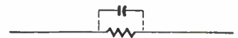
Fig. 4—At v.h.f., a carbon resistor has in effect a capacitor in parallel.
