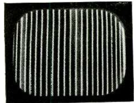
Photo E—Pattern of 23 vertical bars on the receiver screen for horizontal check.
