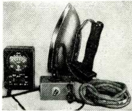
Photo showing the power check setup.
