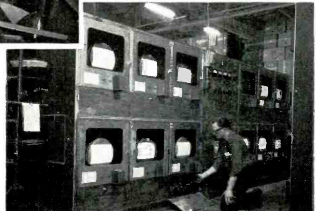
Life testing of large TV tubes is a regular practice. These tubes are run day and night under their maximum ratings.
