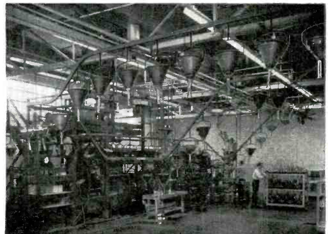
Overhead conveyors and other automatic equipment provide a continuous efficient movement of tubes during production.
