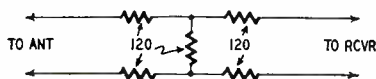
Fig. 4—Circuit for an antenna pad to attenuate a signal that is too strong.
