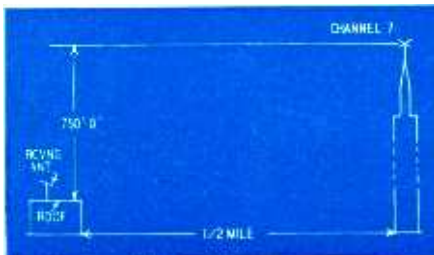
Fig. 1—A receiving antenna near the transmitter but at a much lower level presented a problem of installation.
