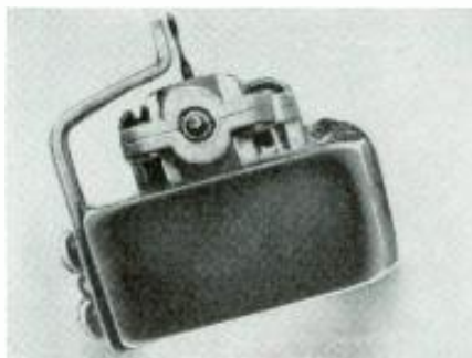
Fig. 4—This head-on view shows separation of the needle and copper strip.
