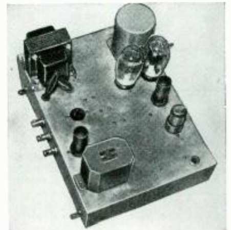
Parts must be mounted so as not to interfere with the turntable motor above.
