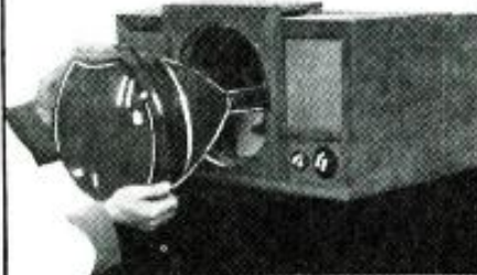
The "All-Vue Corrector" lens being installed in standard set—requiring no electrical changes.
