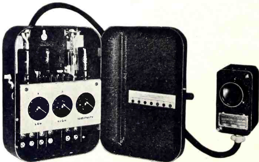
Fig. 4. Photoelectric temperature control with push button.
