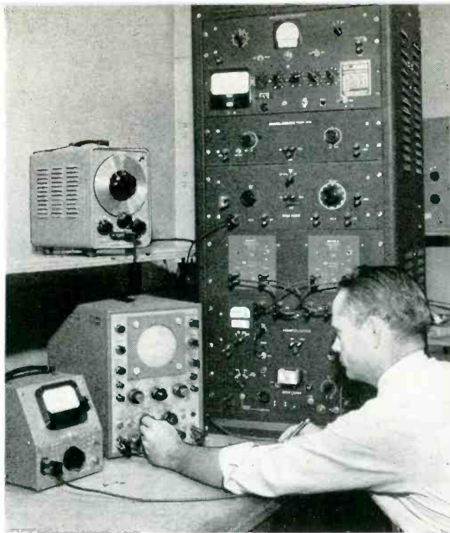
Fig. 1. The test set and auxiliary equipment being used to measure the characteristics of junction transistors.
