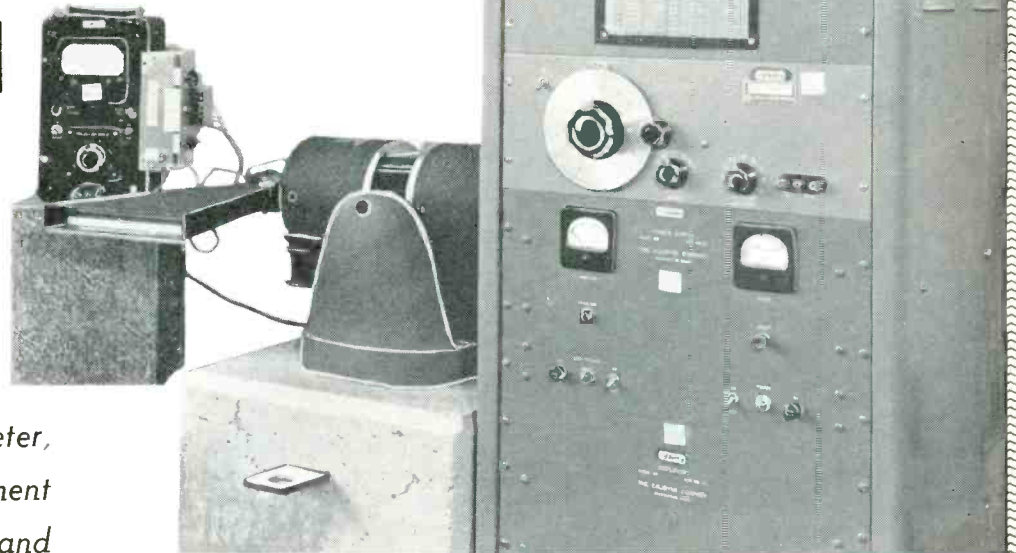
Typical accelerometer calibration setup; Calidyne shaker is positioned horizontally to show optical displacement system.
