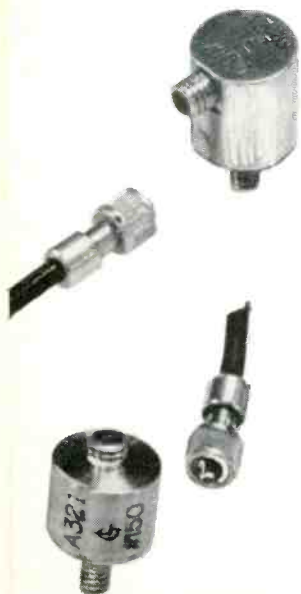
Two miniature vibration accelerometers of the piezoelectric type, typical units which require calibration on a shaker.
