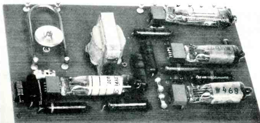
Fig. 10. An experimental superregenerative receiver with printed circuit subminiature sockets. The Auto-Semby technique was used for circuit fabrication.
