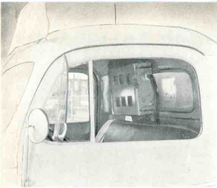
RCA Citizens Radio mobile unit installed in cab of soft drink delivery truck. Dispatcher can contact driver instantly.
