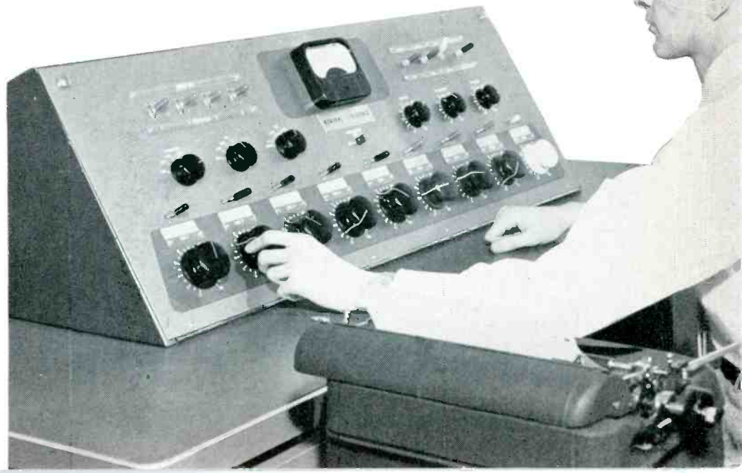
Fig. 1. The G-E BC-11-A broadcast audio console, which uses the plug-in preamplifiers and amplifiers described in the text.
