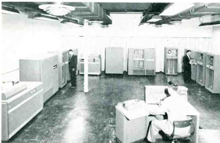
Partial view of the many interconnected units making up the Type "702."
