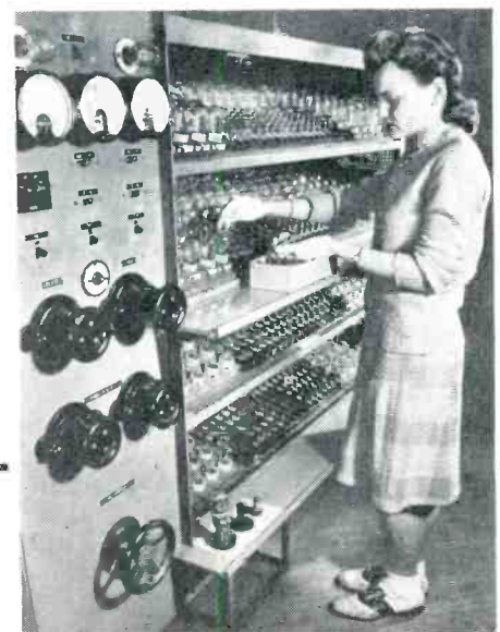
RCA special aging rack for miniature tubes.
