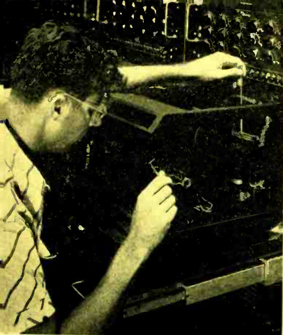
A technician is adjusting the position of a galvanometer in the oscillograph.
