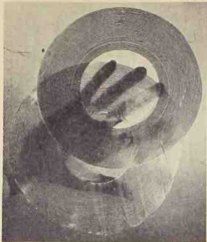
Fig. 3. Samples of etched broadcast loop antennas on plastic film.
