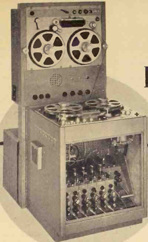
Fig. 1. Commercial laboratory signal-analysis reproducer, Ampex Model S-3037, has 3-speed drive, 8-track reproduction.
