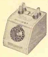
MODELS A, B, & C HELIPOTS A—10 turns, 46" coil, 1-13/16" dia., 5 watts—resistances from 10 to 300,000 ohms. B—15 turns, 140" coil, 3-5/16" dia., 10 watts—resistances from 50 to 500,000 ohms. C—3 turns, 13-1/2" coil, 1-13/16" dia., 3 watts—resistances from 5 to 50,000 ohms.
