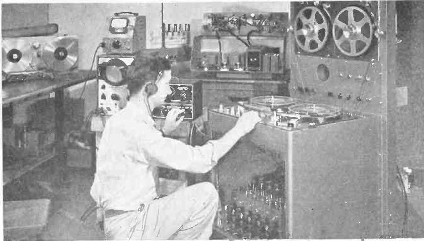
Some form of magnetic recording may solve the problem of recording TV frequencies. Here is some Ampex tape recording and reproducing equipment in use.
