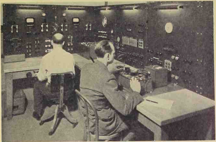
Laboratory at the National Bureau of Standards for testing all types of ammeters, voltmeters, wattmeters, and other electrical indicating instruments.
