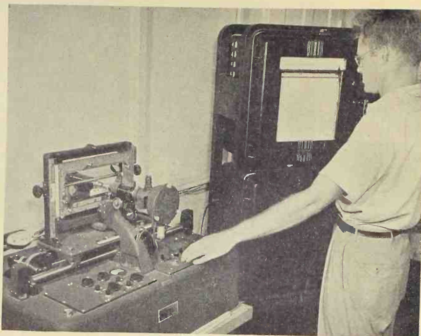
Calibration of Mueller bridge. Accuracy of a few parts in a million may be maintained.
