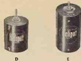
MODELS D AND E HELIPOTS Provide extreme accuracy of control and adjustment, with 9,000 and 14,400 degrees of shaft rotation. D—25 turns, 234" coil, 3-5/16" dia., 15 watts—resistances from 100 to 750,000 ohms. E—40 turns, 373" coil, 3-5/16" dia., 20 watts—resistances from 200 ohms to one megohm.
