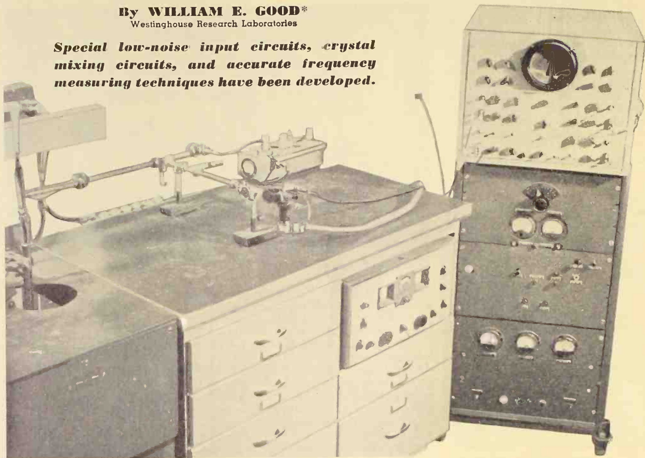
Fig. 1. A portion of the microwave spectroscope including the oscilloscope, the klystron and its power supply.
