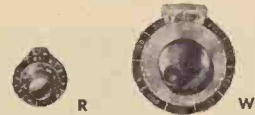
MODELS R AND W DUODIALS Each model available in standard turns-ratios of 10, 15, 25 and 40 to 1. Inner scale indicates angular position of HELIPOT sliding contact, and outer scale the helical turn on which it is located. Can be criven from knob or shaft end. R—2" diameter, exclusive of index. W—4-3/4" diameter, exclusive of index. Features finger hole in knob to speed rotation.
