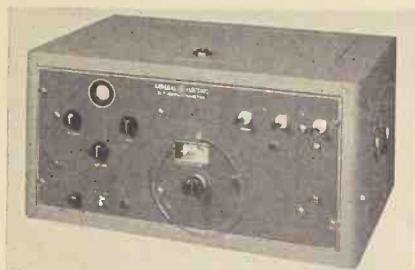
Photograph showing front panel arrangement of the original capacitometer.
