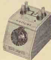
MODELS A, B, & C HELIPOTS A—10 turns, 46" coil, 1-13/16" dia., 5 watts—resistances from 10 to 300,000 ohms. B—15 turns, 140" coil, 3-5/16" dia., 10 watts—resistances from 50 to 500,000 ohms. C—3 turns, 13-1/2" coil, 1-13/16" dia., 3 watts—resistances from 5 to 50,000 ohms. — Ask for Bulletin 104 —
