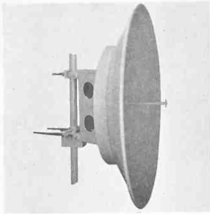
Fig. 2. One of the major advantages of the use of microwaves is that the energy can readily be "beamed" by dipole fed parabolic antennas like the one shown.
