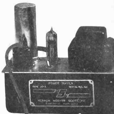
Noise generator and power supply made by H. H. Scott, Inc.
