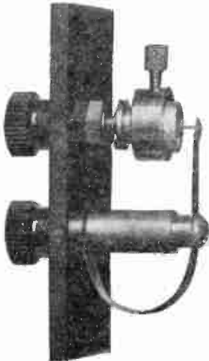
Neutroflex Transformer mounted on Kilbourne & Clark Condenser
