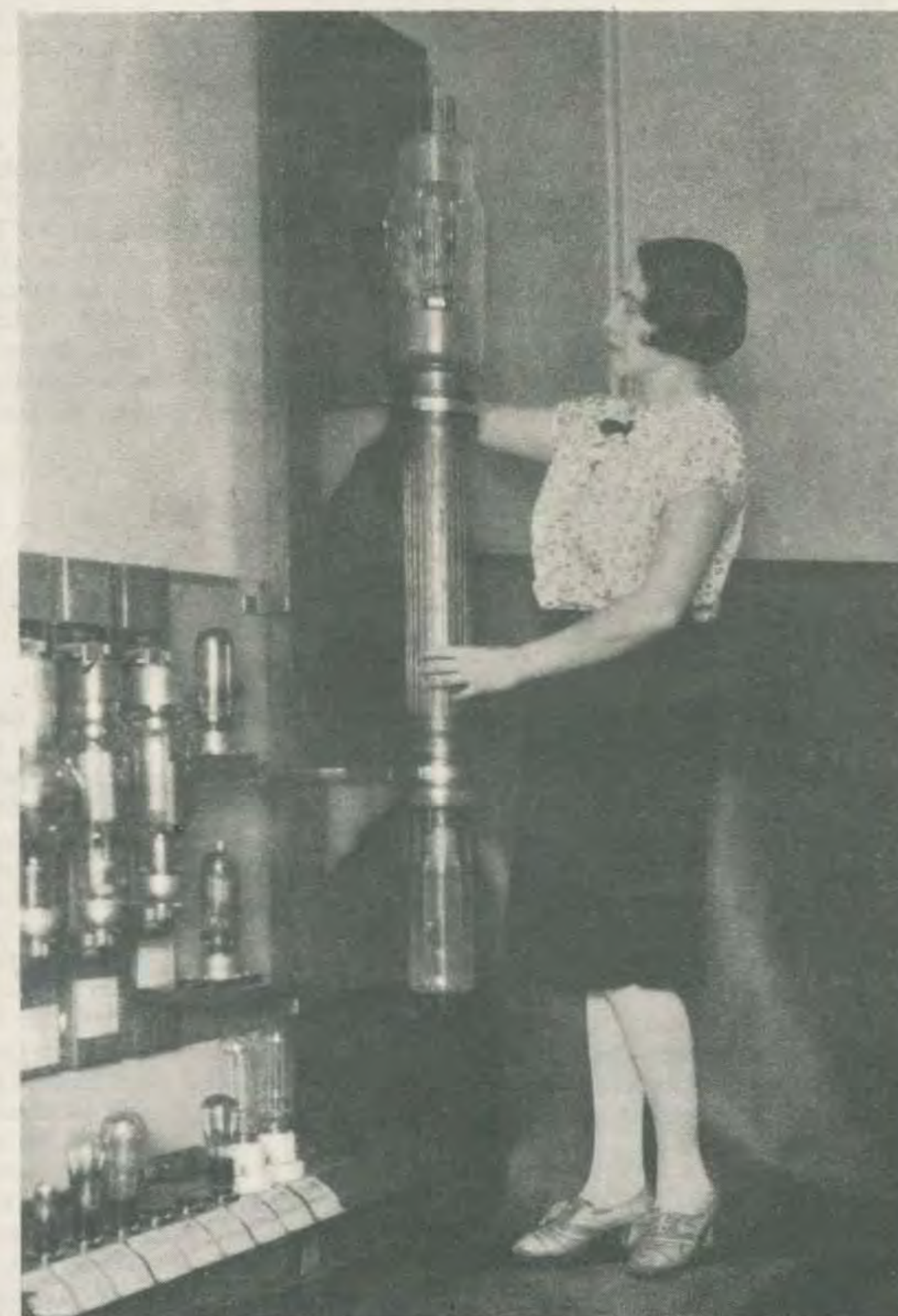
The new tube, designed by engineers of the Westinghouse Electric and Manufacturing Company, to be used in experiments with high power at the new KDKA station being erected at Saxonburg, Pa. This monster tube is six feet tall, weighs 60 pounds, and is cooled by five tons of water each hour of its operation!
