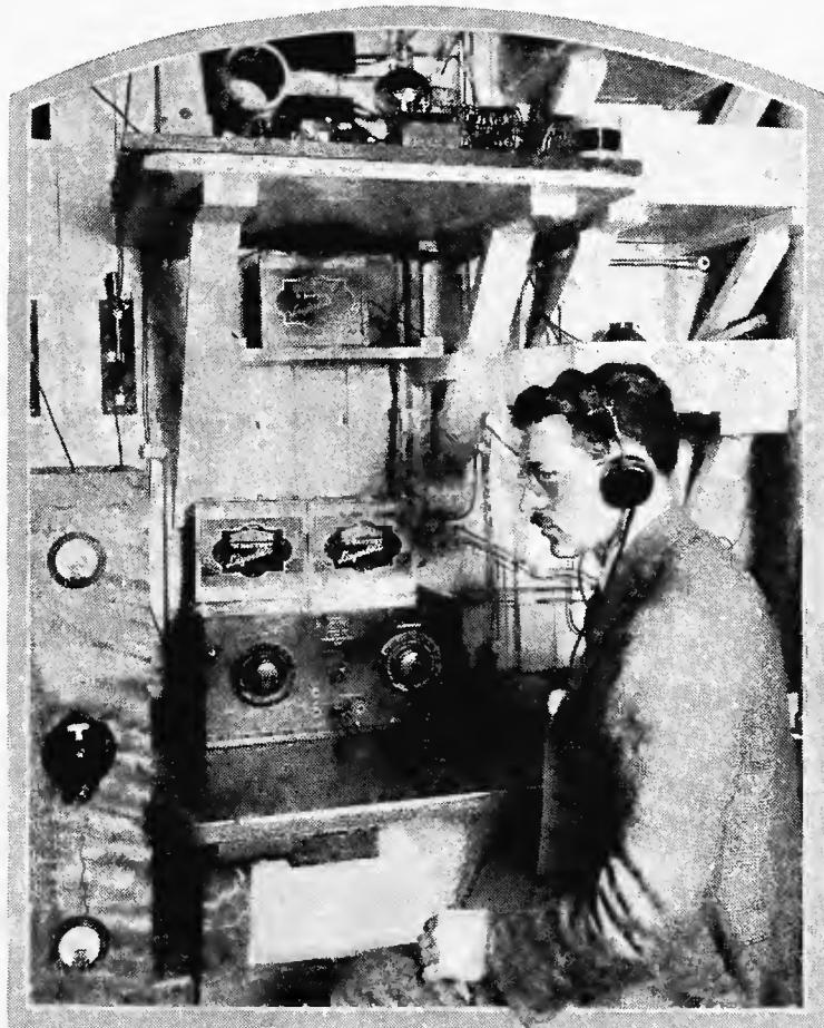
EDWARD MANLEY is shown above at his Radio receiving and transmission sets, aboard the Ed Morrissey , commissioned to carry the Putnam-Baffin Island Expedition into the Arctic in search of the magnetic pole. They will visit regions hitherto unexplored by white men and report back to civilization through short and long wave transmitters. The generator power transmitter is shown at left and the battery powered transmitter with UX 852 tube is shown on the shelf above. The latter has four Radio frequency chokes. The circuit is shown as a tuned plate and tuned grid circuit, for use on 33 and 20 meters. Twenty B batteries supply 900 volts as power. Mr. Manley believes this equipment will be ample to keep the Morrissey in constant touch with New York and the rest of America.
