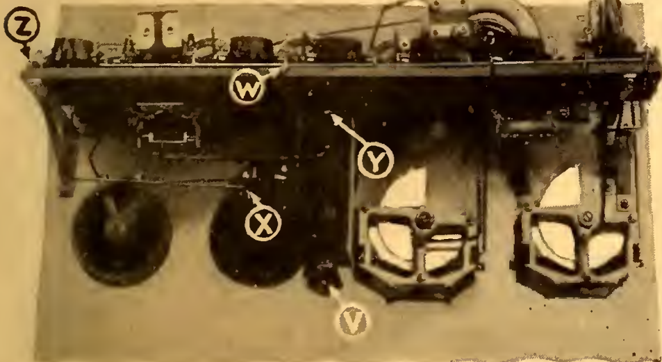
Battery and Speaker Connection Points.
