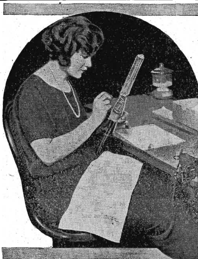
A girl's deft fingers formed the tongue with which S. S. Leviathan "speaks" at will by Radiotelegraph to either side the ocean. Miss Marie Frowick is seen assembling the "tongue" of a 10,000-watt vacuum tube. Two of these furnish the power to the Leviathan's big Radiotelegraph transmitter which has power enough to span the Atlantic. Western Electric Photo
