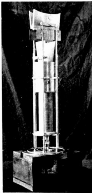
Figure 4. (Above) Machine for grinding and polishing glass covers for 31-inch TCR tube described by I. G. Maloff in his article on page 43, "Direct-Viewing Type Cathode-Ray Tube."
