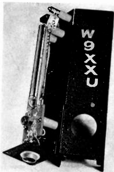
Figure 2. (Top left) The transmitters uncased. Note tuning condenser next to socket.
