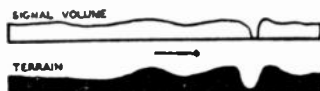
Typical effect of terrain on the volume of received signal. Arrow shows direction of flight.
