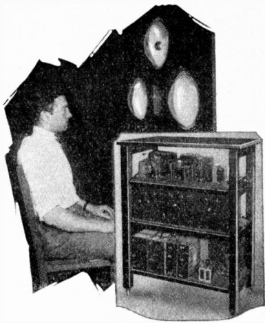
Fig. 1. E. Manuel, sitting before the television transmitter. The insert is the transmitting amplifier. Right, the combination television and broadcast receiver.
