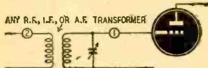
Fig. 4—A quick check method for r.f. coils.
