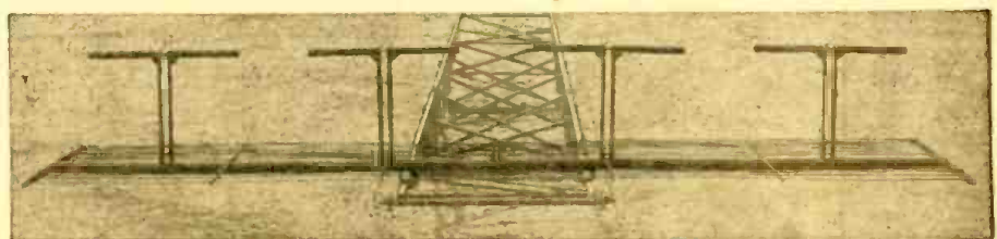
Photo B—A simple horizontal four-element colinear array with a wire-screen reflector.
