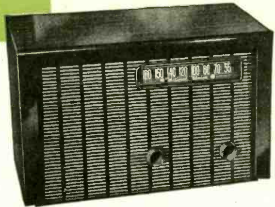
COMPANION MODEL No. 571. 5 Tubes. AC-DC. Superheterodyne Circuit. Built-in Antenna. Automatic Volume Control. 2-Gang Air Condenser Tuning. Illuminated Slide-Rule Dial. Standard American Broadcasts. Walnut Veneer All-Wood Table Cabinet, 13 \frac{1}{2} " x 7 \frac{1}{8} " x 8 \frac{1}{4} ".
