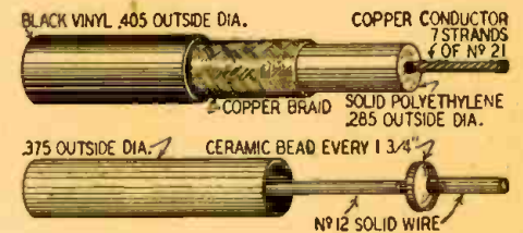
Fig. 6—Two types of popular co-axial cable.
