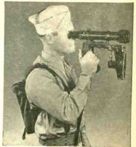
The portable Snooperscope and power supply. A modified form of the instrument, called a Sniperscope, attaches directly to a carbine.
