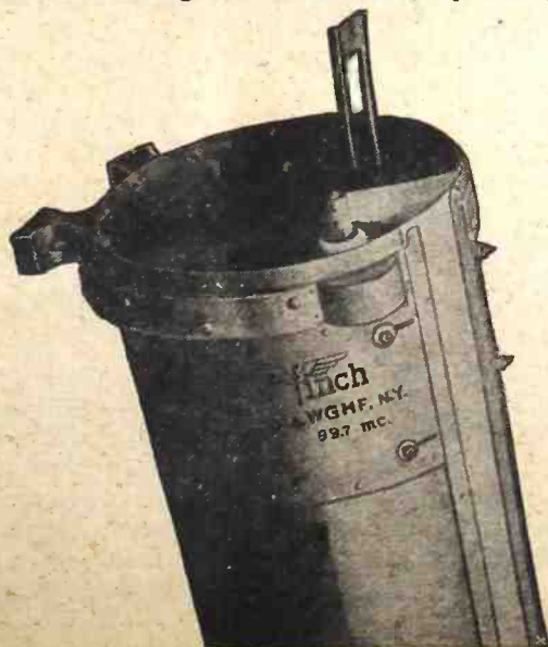
Close-up view of the new facsimile antenna.
