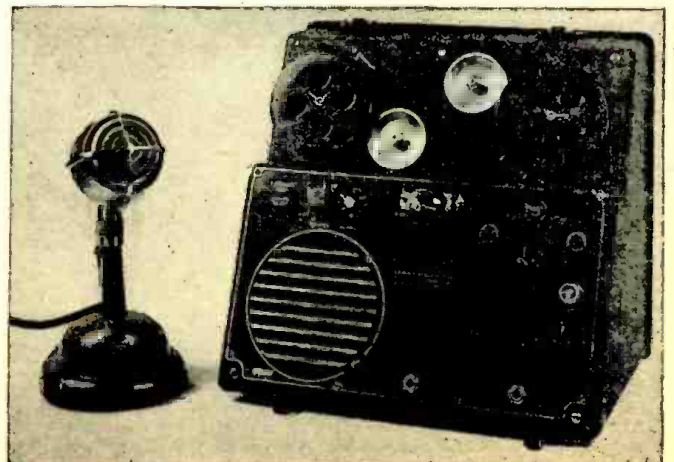
The original Model 50 wire recorder, used extensively during the war, appears at the right. Its ruggedness gave it a marked advantage over less sturdy types of recorders. At left is a magazine model, with the magazine shown lifted just clear of the sockets into which it fits.
