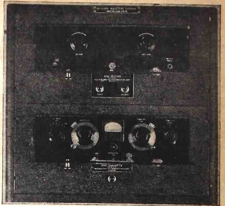
A Zone transmitter (bottom) and receiver (top). There are only two receiver controls, R.F. and audio gain.
