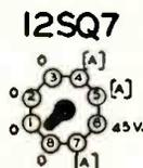
\* OSC. VOLTAGE TO BE MEASURED WITH R.F. CHOKE IN SERIES WITH VOLTMETER LEAD.
