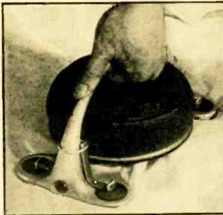
Photos above show front and side views of the Penetron sound reproducing instrument; it is held to the glass of a store window by vacuum cups as indicated. Photo below—How easy it is to place the Penetron into a new Location—the rubber vacuum cups lock it in position.
