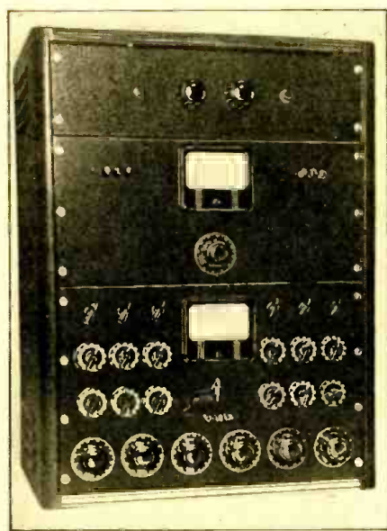
Fig. 1. The completed Semi-Professional Recording-Playback Amplifier. Identification of the equipment on the 3 panels (reading from left to right): Top Panel: "B" supply pilot and switch; "A" supply switch, and pilot. Middle Panel: off-lip of triodes Nos. 1 and 2; power level VU meter; off-plus 30 VU and 40 VU; (center knob) amplifier gain control. Bottom Panel: consider these controls in vertical rows, the first 5 of which are channel controls, bottom to top, as follows: channel volume control, L.F. control, H.F. control, dialogue filter switch. Row 6: master volume control, monitor volume control, expander control, expander-compressor switch. The meter is a vacuum-tube VU type; underneath is the VU range selector switch; the 3 buttons underneath read: Monitor, Recording and Playback.
