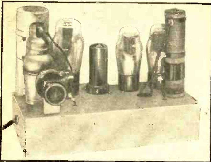
← High-gain, high-power A.F. amplifier, complete with voltage multiplier type of power supply designed to deliver high voltage without requiring the use of a step-up transformer.
