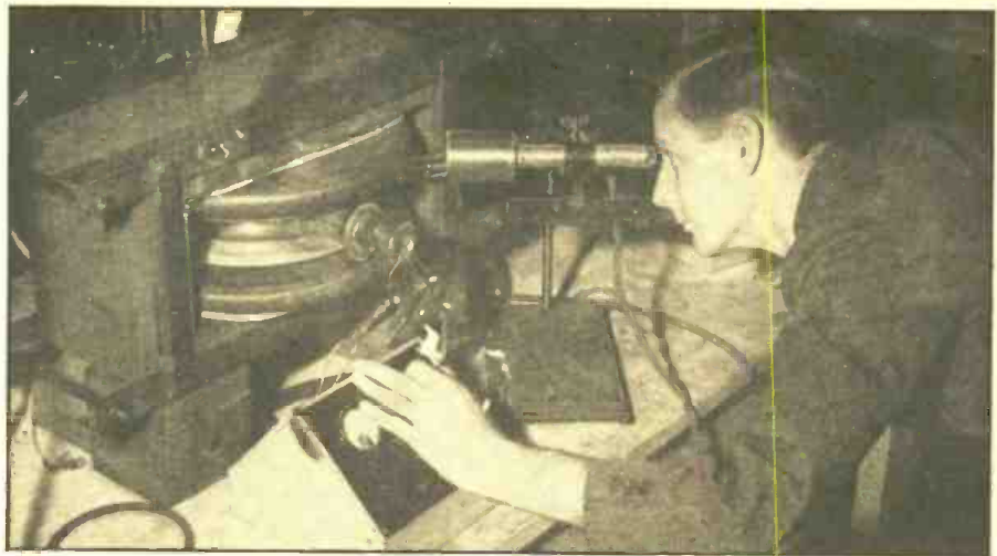
Electroscopic study, of the radiations by the "Acceletron," or Induction Electron Accelerator, by Dr. D. W. Kerst of the General Electric Research Laboratory. The "spot" illustration on the cover of Radio-Craft shows Dr. Kerst examining the doughnut-shaped vacuum-tube—or "race-track" for electrons—in which electrons gain almost the speed of light; and develop millions of volts for use in atom-smashing and other fundamental physics experiments.
