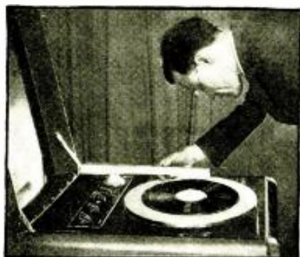
Here an operator is shown using the new 9A pickup as a part of the 1300A sound-on-disc equipment. The pickup by exerting a pressure on the record of only about 30 grams (0.9-oz., approx.), minimizes record wear and stylus noise. The diamond stylus has practically unlimited life. The output rating (equalized) is about -70 db.
