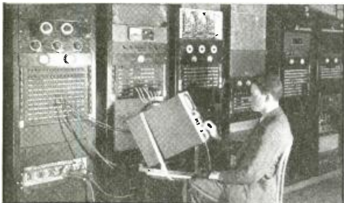
Amplifying and control equipment of the stereophonic system. A. R. Soffel of Bell Telephone Labs. is shown observing the channel levels on a cathode-ray tube monitor.
