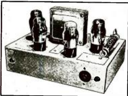
Fig. 1. Completed rectifier; extreme right, tapped keying bleeder connected across the output.
