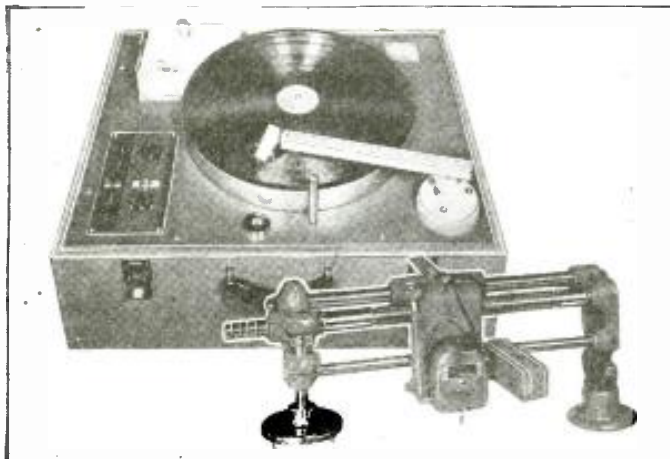
At left is shown the RCA model MI-4814 Turntable for making high-quality recordings even on transcription-size discs 16 ins. in dia.; the leadscrew and cutting head are shown at lower-right. Instrument has heavy, rim-drive table; records at 78 or 33 1/3 r.p.m.; used with any available recording amplifier. Cutting mechanism is removable as shown. Has magnetic cutter, and magnetic
