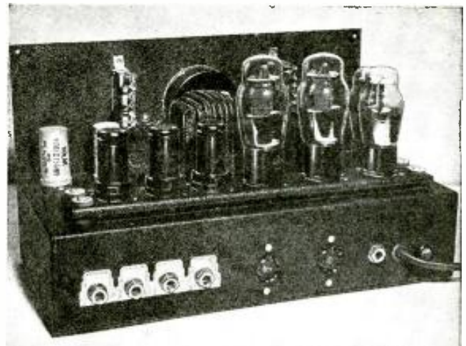
The amplifier rear view, above, shows the tubes mounted on an anti-microphonic base. Unit includes the following features: Variable high and low inverse frequency compensation with concentric constant-current inverse feedback inverter; humless push-pull beam power output; dialogue filter; low-level, noiseless, non-frequency discriminating gain controls (adapted for remote control).
