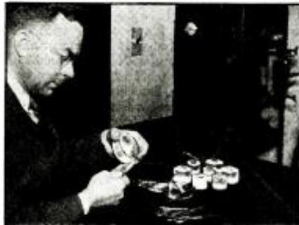
Here Professor Stockbarger is shown removing a 3-inch crystal of lithium fluoride from the thin platinum crucible in which it was artificially-grown at a temperature of more than 1,200° Centigrade. Before him are other crystals of various sizes. The electric furnace in which they were grown is shown at the right. Next step is cutting and polishing the crystals.
