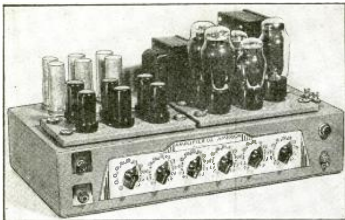
Fig. A. View of the 30-W. direct-coupled amplifier with variable expander feature included.
