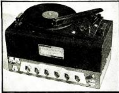
Front view of the neutralized-feedback amplifier. Its various controls, from left to right, are: Microphone No. 1 Volume; Microphone No. 2 Volume; Phono Volume; Auxiliary Input Volume; Low-Frequency Tone Control; High-Frequency Tone Control.
