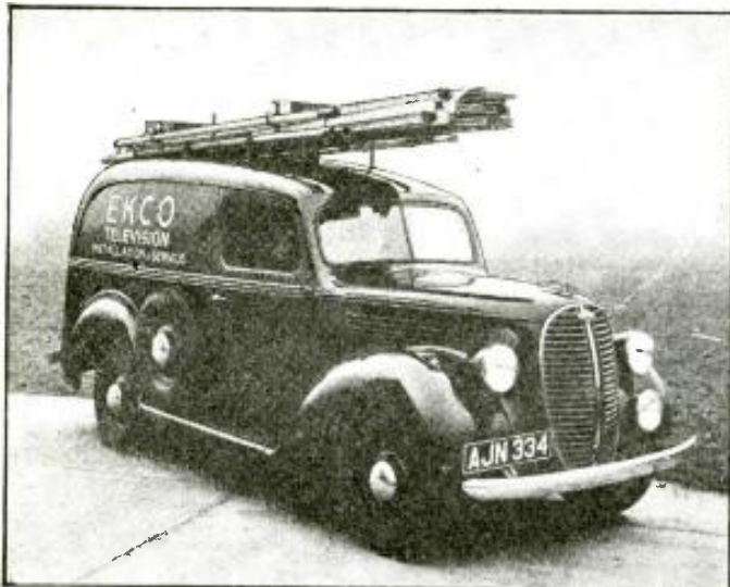
The English manufacturer, Ekco, has produced the television service car illustrated above for use in London and environs. Every device required by the Serviceman for the installation and maintenance of television receivers is on hand. An extensible ladder is topped by a television antenna.
