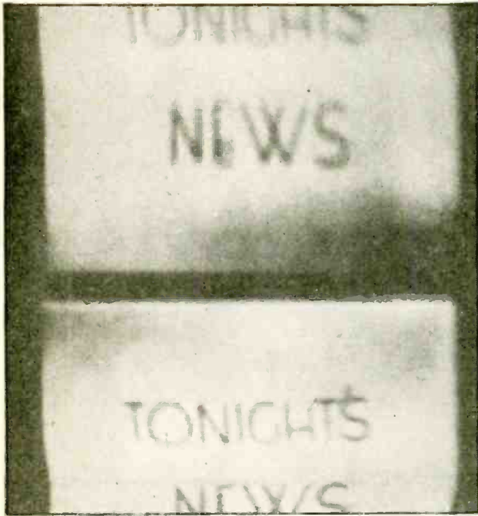
Fig. 4. Frame time base operating at \frac{1}{2} the correct frequency.
