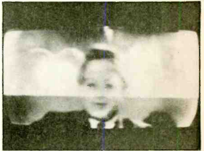
Fig. 5. Frame time base operating at twice the correct frequency causes the image to overlap.
