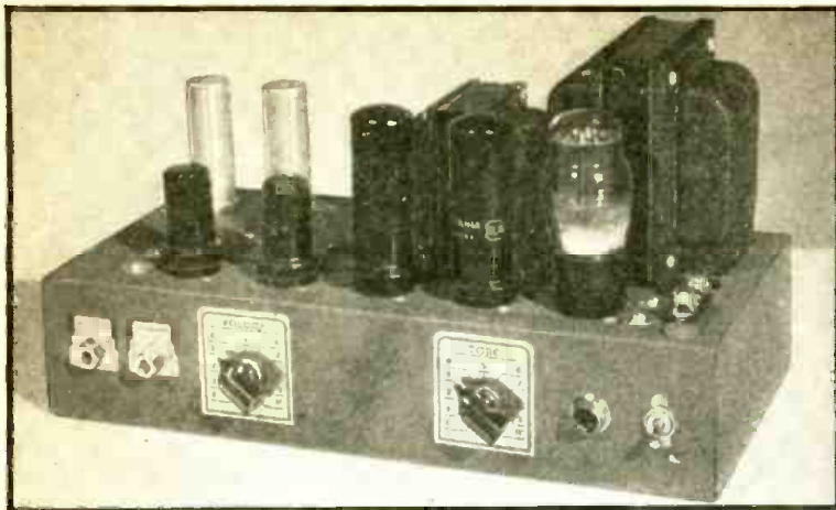
The 10-W. All-Push-Pull Direct-Coupled Amplifier. Note its simplicity, and compactness. A view underneath the chassis will amaze you with its scarcity of components.
