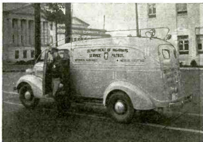
STATION KACW, mobile unit for rendering medical first-aid, mechanical assistance on the highway, cooperation with the police and fire departments, and other services. It has both receiving and sending equipment.
