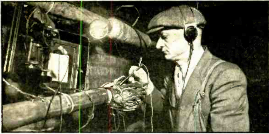
Ladies and gentlemen—meet Bell Tel. Co.'s "bliffy sniffer"! Nearly as we can make out, the "bliffy" is an amplifier and the "sniffer" is a prod which noses-out a "live" wire. In old system, a tone put out a wire (one of a number in a telephone cable under test) at a remote point was "buzzed-out" with earphone and contact prod until tone was heard. In new scheme, prod merely comes near the wire.
