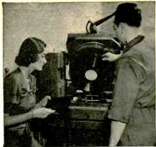
9 —PRESSING MACHINE—Now we start making records. Disk goes into a hydraulic press, and a "biscuit" of plastic material is put next to it. Comes a ton of pressure—and the result is a perfect duplicate of the original wax recording.
