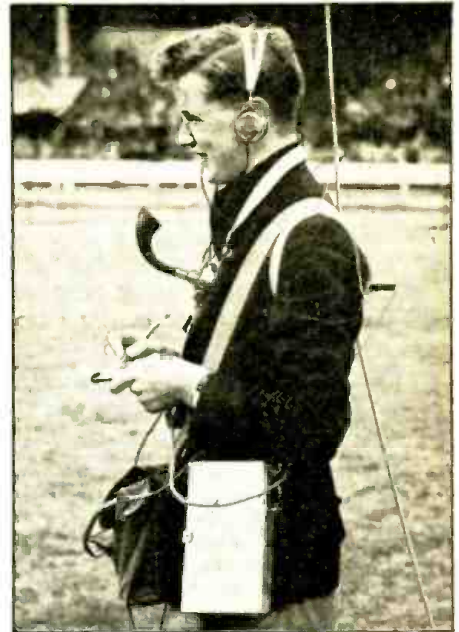
The Annual Amateur Athletic Association Championships held recently at White City, London (Eng.), inaugurated the use of a pack transmitter to radio the results to the scoreboard control.
