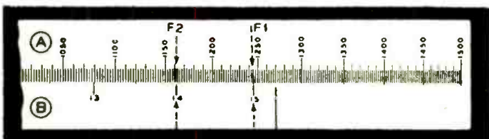
Fig. 4. Dial calibration procedure. With receiver dial set, vary adjustment of test osc. until 2 different signals are received; say, F1 = 1,245 kc., and F2 = 1,162 kc. Slide rule until 2 harmonic numbers coincide, for example— \frac{1,245}{15} and \frac{1,162}{14} . If 1,245 \times 14 = 1,162 \times 15 frequency of dial calibration is established.
