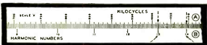
Fig. 5. Aligning high-frequency bands. Example: (Assume alignment desired at 14.2 mc.) (1) Divide 14.2 mc. by some usable harmonic number say 13. 14.2 \text{ mc.} \div 13 = 1,093 \text{ kc.} (2) Add one unit to harmonic number 13 + 1 = 14 . (3) Slide scale "B" until 14 coincides with 1,093 kc., and 13 coincides with 1,015 kc. (4) Adjust high-frequency trimmers until a signal is received at 14.2 mc. dial setting when osc. is alternately tuned to 1,015 kc. and 1,093 kc.
