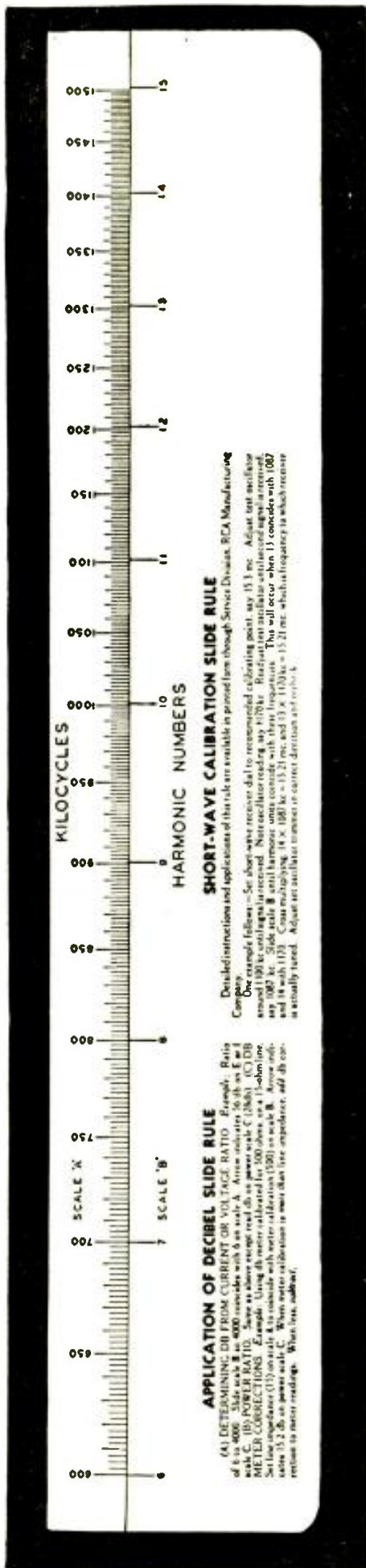
Fig. 2. Reverse side of RCA 9 7/8 x 1 3/4-in. sliderule.
